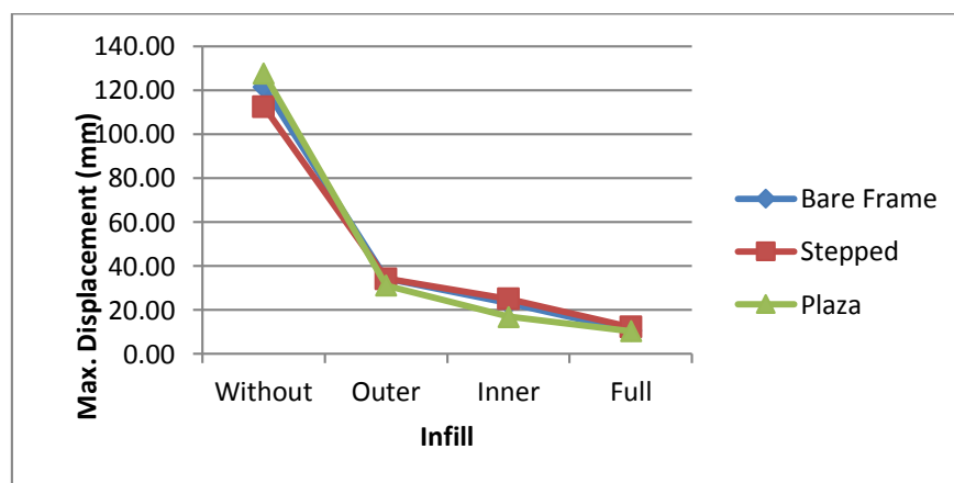
Fig. 5: Maximum displacement in X direction with cement brick infill
